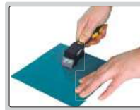
step 1: make grid cutting on surface
