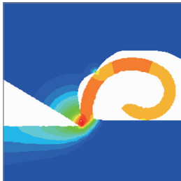
New tooth design with chip breaker
