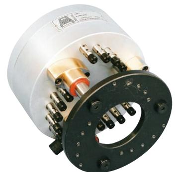
*components are hardened and ground, and are carried in anti-friction bearings enabling these heads to run up to 10.000 rpm. In special cases, MT heads are built with large bodies and high numbers of spindles - even in excess of 20.*
